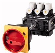
**Main switch, P5, 125 A, rear mounting, 3 pole, Emergency switching off function, With red rotary handle and yellow locking ring, Lockable in the 0 (Off) position**
