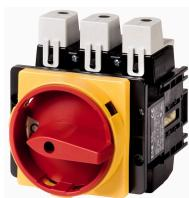
**Main switch, P5, 125 A, flush mounting, 3 pole, Emergency switching off function, With red rotary handle and yellow locking ring, Lockable in the 0 (Off) position**
