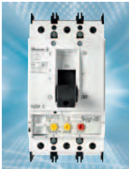
Figure 3: The motor protective circuit breaker NZM2-ME-NA, listed per UL 489 and certified per CSA-C22.2 No. 5-02, has additionally been evaluated per the motor overload calibration requirements of UL 508 and CSA-C22.2 No. 14. In addition to the adjustable overload and instantaneous short circuit trip adjustments, the device has a motor inrush trip class selection feature similar to the ones available in premium design overload relays.
