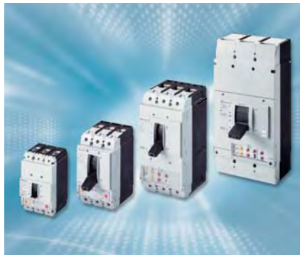
Photo 3: Modern current limiting Molded Case Circuit Breakers Type NZM with short circuit interrupting ratings established per the North American norms at levels up to 100 kA rms sym @ 480VAC and 50 kA rms sym @ 600VAC.
