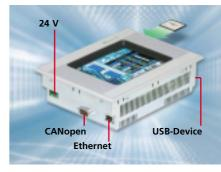
The XVH-340 (IR Touch) and XVH-330 (Resistive Touch) are specially developed, high-performance low-budget data management and visualization systems with Ethernet and CANopen on-board. They are used mainly in the fields of machine engineering and industrial automation.
