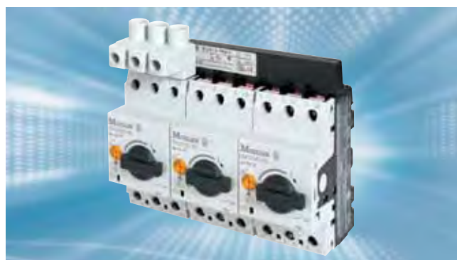
Photo 12: 3 UL 508 Type E- Motorstarters (Manual Type E Self-Protected Combination Motor Controller), shown here as a small grouping with bus link connectors for use e.g. in a decentralized automation process. Of particular interest is the large spacing terminal block BK25...-E, which in this particular array would only need to be used once to provide the larger electrical clearances for the incoming supply. This terminal must be provided on each individually equipped motor starter adapter destined for export to North America.
