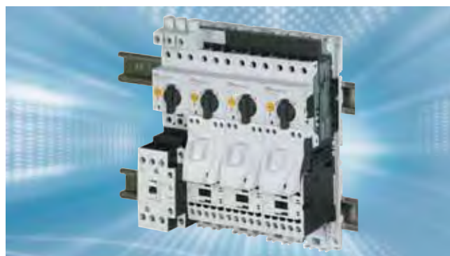
Photo 13: 4 UL 508 Type F- Motorstarters (Type F Combination Motor Controller), shown here as a small grouping with bus link connectors mounted on DIN (mounting) rails, are made up of self-protected manual motor controllers combined and tested with a magnetic contactor. Type F-Motorstarters can also be mounted on busbar adapters, in which case the large spacing terminal block BK25...-E would be required for each starter branch when exporting to North America.
