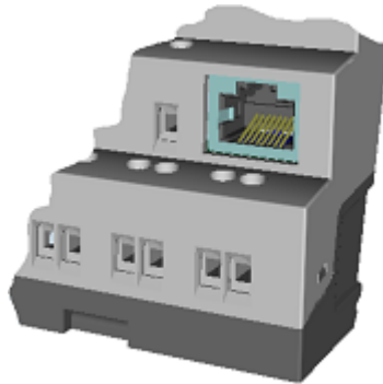
Abb. 32: RJ-45 Buchse, 8-polig
