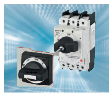
Photo 8a: The new supplementary handle for Frame size 2 switches. The well-established door mounted rotary handle, which operates the switch with the door in the closed position, appears in the foreground.
