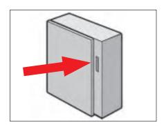
Photo 5: Typical North American enclosure with a flange mount and opening on the side to allow for "vertical motion" handles.
