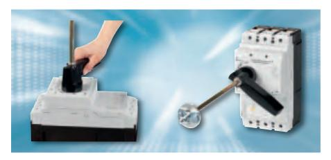
Photo 9: A larger version is necessary to adequately handle the greater forces required to switch the larger frame sizes NZM 3 and 4. An identical "deliberate action" feature consisting of an initial travel followed by simultaneous pushing and turning motion applies to this handle as well.
