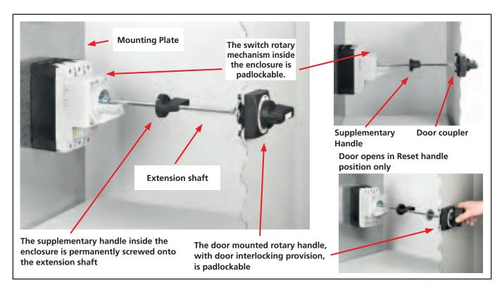
Photo 1: Former solution with older version supplementary handle, lockable rotary switch mechanismand lockable door mounted handle.
