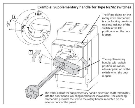
Photo 8b: The new supplementary handle NZM....XHB-DA(R)-NA requires a deliberate action (by qualified persons) before it can be engaged to operate the switch to the ON position, should the control panel door be open (e.g. for maintenance purposes). The deliberate action consists of the following 3 operational movements:
