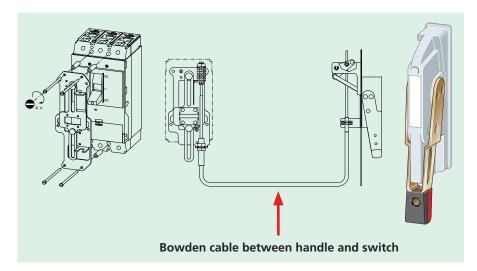
Photo 6: The vertical motion handle (right) depicts the typical North American main disconnect switch handle which, independent of the door position, remains in contact with the switch. The use of flexible, Bowden cable solutions is more often encountered in control panel applications. The handle and enclosure also combine to mechanically interlock with the door.
