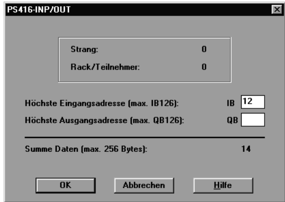
Figure 2-5: Parameter setting of the PS416-INP-400/-401
